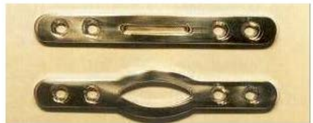
Figure 3 – This NiTi bone plate has been heat treated such that the central part changes from its deformed shape (top) to its memory shape (bottom) when warmed with saline solution, thus drawing the two ends of the fracture closer together. The modulus of this material has also been closely matched to that of human bone. (Courtesy of Tony Anson, Anson Medical Ltd).
